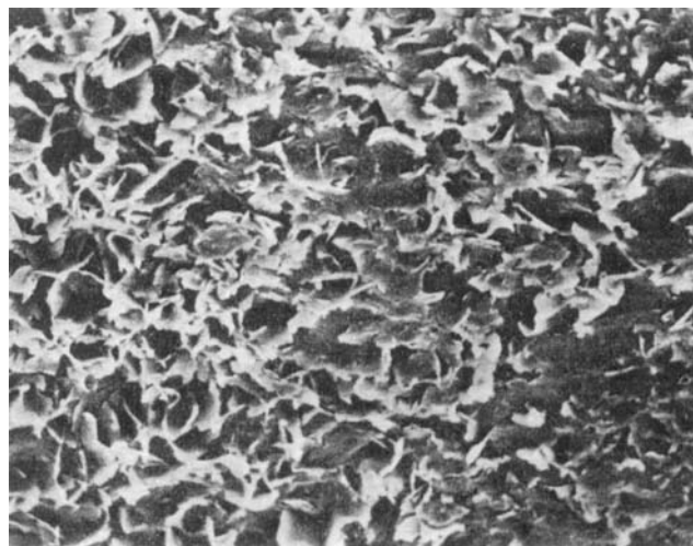
Figure 7 —Electron scanning micrograph of the surface of a stearyl alcohol particle encapsulated by the modified method (magnification about 500 \times ).
